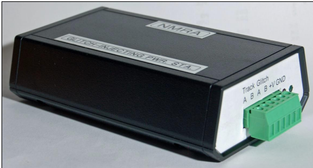
Figure 9: Completed Glitch-Injecting Power Station
